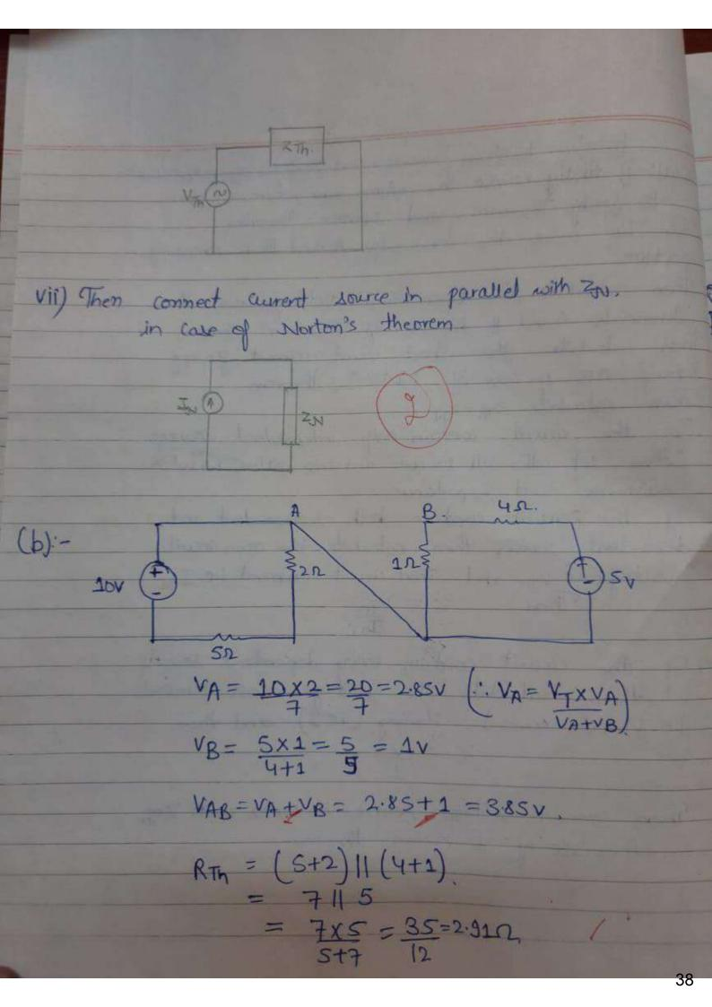
RT = 2-9112. MH=3.82 (~ VS:ms:- (a) voltage source, resistance is converting into by connecting a resistance parallel to current source and value of current source in by I = V. Conversion of voltage source into current source  $\Rightarrow \bigoplus_{\mathbf{r}} \mathbb{I}_{\mathbf{r}} \mathbb{I}_{\mathbf{r}}$ current source. voltage source (b) Filters: - Filters are used to got an pure DC outpart from pulsating Dic and are used to filters out got oscillations from output:
